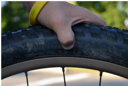
While checking for air pressure, riders should also inspect their tires for damage and wear.
